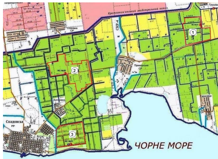
Figure 1 – pump stations are investigated in the rice irrigation systems 1 (PS №13) - Hrushivska rice irrigation system; 2 (PS №20) - irrigation system under ДФ-120 "Dnipro"; 3 (PS №21) - the Closed Check-closed irrigation system by V.J. Makovskiy
